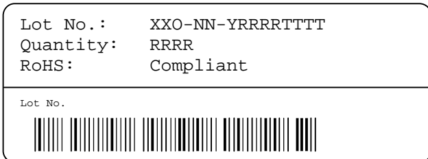
Figure 11: First label on reel: XX = Sensor Type (21 for SHT21), O = Output mode (D = Digital, P = PWM, S = SDM), NN = Chip Version, Y = last digit of year, RRRR = number of sensors on reel, TTTT = Traceability Code.
