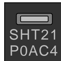
Figure 10 Laser marking on sensor. For details see text.
